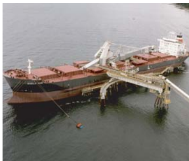
Sechelt ship loader identical to the one being built at Orca Quarry
